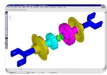
Above: Speakes used Cobalt CAD and 3D modeling software to reverse engineer the Ferrari's missing cam and pawl differential.
