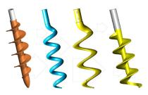
Cobalt 3D models showing from left to right, the first "sand moving tool," the perfect but too expensive steel prototypes and the final injected polypropylene tip.
