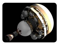
Jones designed the truss structure for the Instrument Deployment and Return Vehicle (IDRV) starting with a rough concept in Graphite precision drafting software, then brought that file into Cobalt modelling software to create and render a full 3D model.
