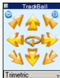
Click on one of the arrows to rotate the view continuously in the selected direction. It will look like it's spinning. To make it stop spinning, click in the drawing area of the screen.
