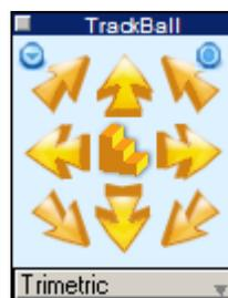
This is the step mode of the Trackball. Clicking on any of the arrows in the window displays the model in increments as it rotates around its point of rotation. The icon in the middle (resembling a staircase) indicates that clicking on the arrow moves step by step. Click on the stair icon to change to an arrow.
